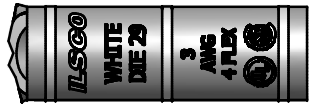
DETAIL A, SCALE 2 : 1 TOP & BOTTOM INK MARKING INK COLOR: WHITE PER SPEC #: F921
