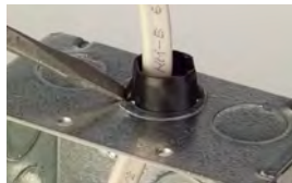
Easy Removal - Push the wing tab of the connector with a screwdriver. Push the connector through the knockout towards the inside of the box.
