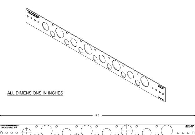
The HOLDRITE #107-18 is a Copper-Bonded<sup>™</sup> steel bracket with holes on 2" centers to position 1/2" copper tubing and holes on 4" centers to position 3/4" and 1" copper tubing.
