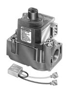
These universal electronic ignition gas controls are used in gasfired appliances with capacities up to 150 cu ft/hour at 1 inch wc pressure drop (4.2 cu m/hour at 0.25 kPa) for natural gas. The VR8245M will operate with a direct spark (DSI), hot surface (HSI) or intermittent pilot ignition. The control includes a manual valve, two automatic operators, a pressure regulator, pilot adjustment, pilot plug and ignition adapter.
