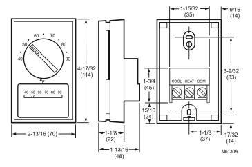
Dimensions, Approximate: 4 1/2 in. high x 2 15/16 in. wide x 1 1/2 in. deep (switches and wiring terminals protrude into outlet box 3/4 in.) (115 mm high x 75 mm wide x 39 mm deep (switches and wiring terminals protrude into outlet box 19 mm))
