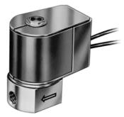
Body Pattern: Straight through Dimensions, Approximate: 2-3/4 in. high x 1-5/8 in. wide x 2-5/8 in. deep (70 mm high x 41 mm wide x 67 mm deep) Current (max amps at rated Vac/Hz): 0.115 amps Power Consumption: 8 W Electrical Ratings: 120 Vac
