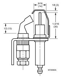
Nonprimary-aerated combination pilot burner and ignitor. Used with the S86, S860, S8610, or S8670 in intermittent pilot systems.
