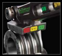
Correctly align the tube size with color-coded indicators.
