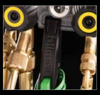
Attach K-style clamps to an easily accessible spot on the hilmor manifold.
