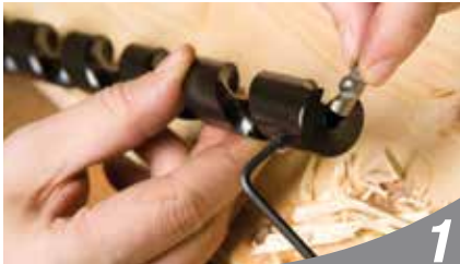
1 Insert Cutting Edge...
