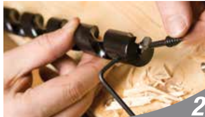
2 Insert Feed Screw...
