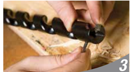
3 Tighten Set Screw.
