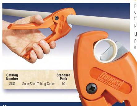
A patented V-point blade pierces hard or soft plastic tubing, then slices through to give a clean, easy cut with virtually no tube deformation. The blade is offset to give you powerful, penetrating action with a minimum of force.
