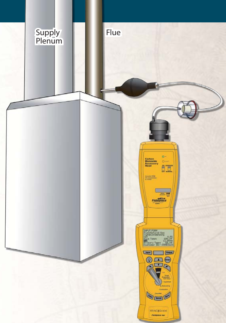
Figure 17. CO measurement of flue gas for the Combustion Test using an ACM3 Carbon Monoxide Head and the pump that's included with the AOX2 Combustion Check Head.
