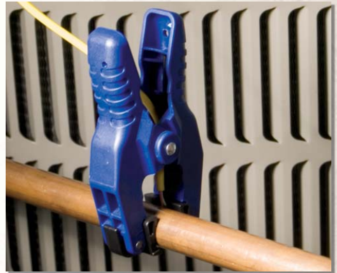
Figure 15. ATC1 pipe clamp thermocouple attached to a pipe correctly.
