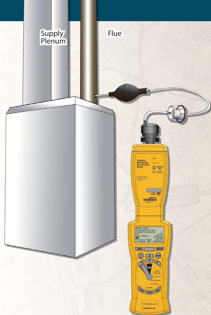
Figure 34. Entering the CO measurement for the Combustion Test using an ACM3 Carbon Monoxide Head and the pump that's included with the AOX2 Combustion Check Head.
