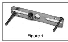
**1.** Assemble two (provided) Threaded Rods on the Crossbar. (Figure 1)
