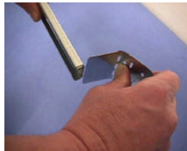
Bend ends of bracket as shown (either 1 1/2" or 2 1/8" box depth)
