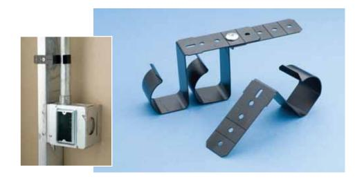
CADDY® Screw-On Conduit Supports from ERICO® securely attach EMT conduit or MC/AC cable to wood and metal studs. The supports comply with NEC® 358.30(A) and CEC® rule 12-1404 which requires conduit support within 36" of an electrical box and also comply with CEC Rule 12-618 which requires support of an armored cable within 12" of an electrical box.
