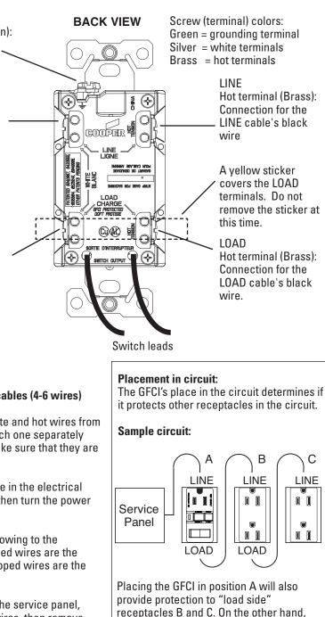
placing the GFCI in position C will not provide protection to receptacles A or B. Remember that receptacles A, B, and C can be in different rooms.
