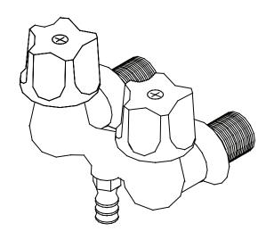
The leg tub fitting has a cast brass body with replaceable seats. The fitting body and spout are polished and chrome plated. The outlet spout is designed for a push on hose connection. The spout fits hose with a 1/2-inch inside diameter. The compression stems are all brass with a double O-Ring seal and rubber seat washer. The canopy handles are zinc die cast with a chrome plated finish.
