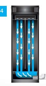
The combustion gases are then forced downward through eight 2" 3rd pass heat exchanger tubes and reach the exhaust collector at a temperature of approximately 120°F.
