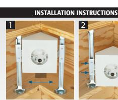
For proper fan/fixture installation, use supplied template to level and position brackets between rafters. Remove captive screws on sides of brackets and use to attach FBX900 assembly to rafters.
