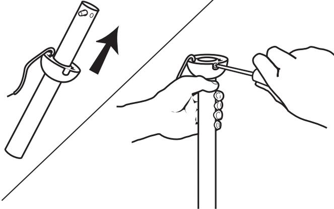
Re-install pin into extended downrod, and slide downrod ball up to the top of the downrod. Re-install set screw to secure ball to downrod. Note: Some extended downrods have a pre-drilled set-screw hole. If a pre-drilled hole is present in the extended downrod, tighten the set screw into the pre-drilled hole in the extended downrod. If no pre-drilled hole exists in the extended downrod, tighten the set screw against the downrod to secure the downrod ball.
