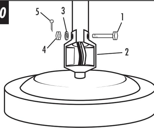
Thread leadwires through the downrod and install crosspin (1) through yoke (2) and downrod. Install lockwasher (3) and nut (4) and tighten. Install cotter pin (5).
