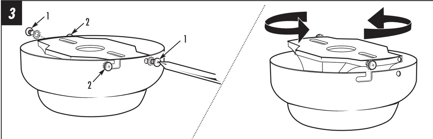
Remove the screws and star washers from the two mating holes (1) on the canopy. Loosen (**do not remove**) the screws in the mating slots (2) on the canopy. Rotate the mounting bracket counter-clockwise and remove from the canopy.
