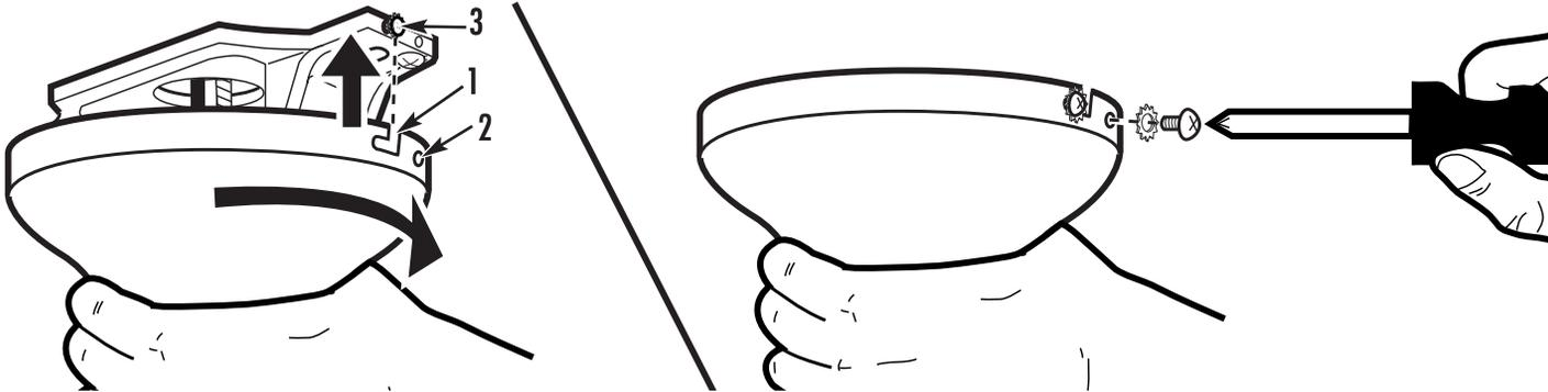
The canopy has two mating slots (1) and two mating holes (2). Position both slots on canopy directly under and in line with two screws in the mounting bracket (3). Lift the canopy, allowing the two screws to slide into the mating slots. Rotate the canopy clockwise until both screws from the mounting bracket drop into the slot recesses. Tighten screws securely. Install two screws and star washers into the mating holes of the canopy and tighten to secure the canopy to the mounting bracket.
