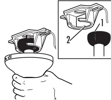
Carefully lift fan assembly onto mounting bracket. Rotate fan until notch on downrod ball (1) engages the ridge on the mounting bracket (2). This will allow for hands free wiring.
