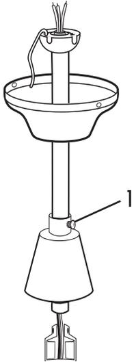
Loosen set screws on the lower canopy (1). Install canopies onto downrod as shown. Thread lead wires through the downrod.
