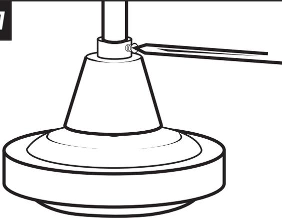
Loosen set screw in lower canopy and slide to within 1/4" of the motor. Tighten set screw(s) in the lower canopy. Make sure there is at least 1/4" clearance maintained around the motor and lower canopy.
