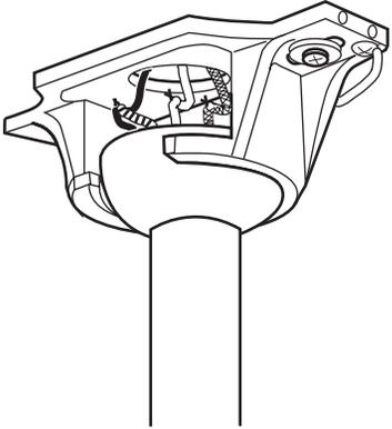
With bracket holding fan assembly, make electrical connections using the following step for wiring instructions.
