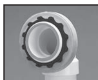
Easily remove membrane after test
